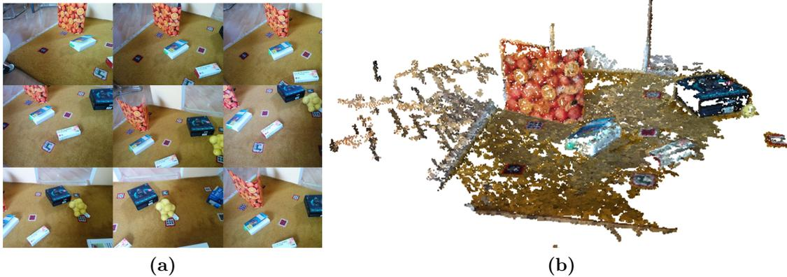
**Figure 4.2:** Scene *Carpet*. (a) shows nine out of twelve input keyframes. (b) shows the reconstructed scene. A densification algorithm like PVMS[24],[23] is applied to the sparse 3D point cloud.
