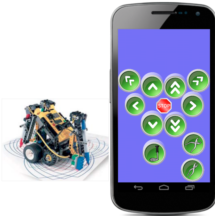
Figure 4.4: Catroid while executing a program to control Lego Mindstorms robots [19]
