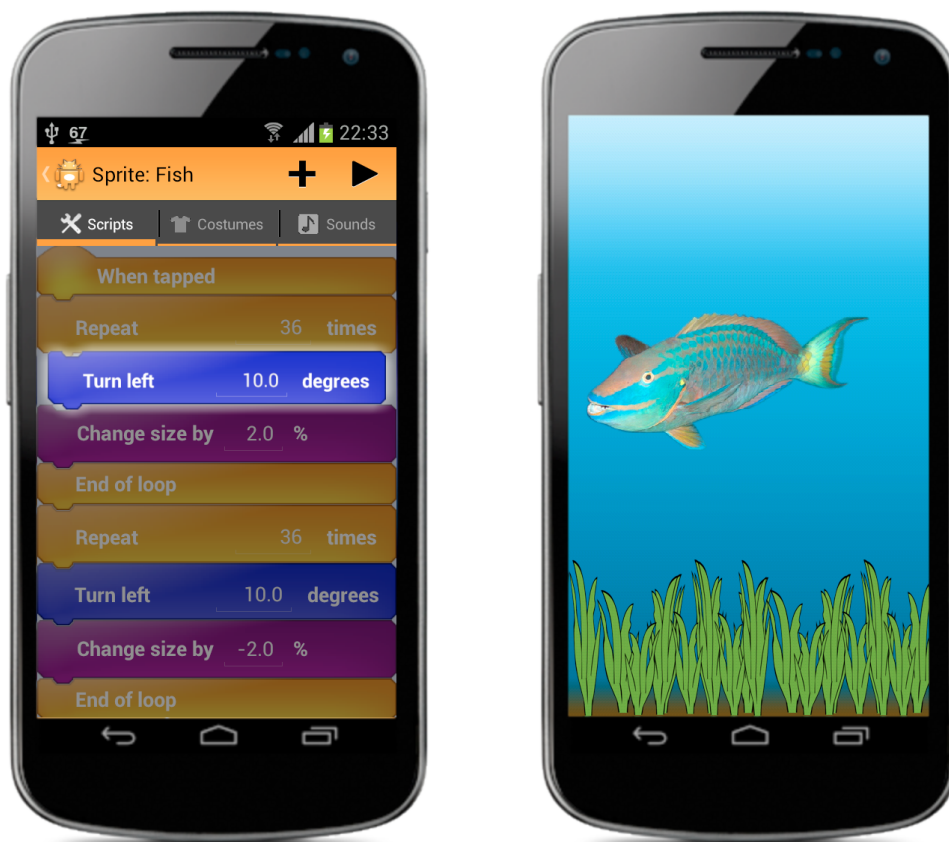
Figure 4.2: Catroid in Action: The left image shows Catroid while creating a program. The right image shows Catroid while executing this program.
