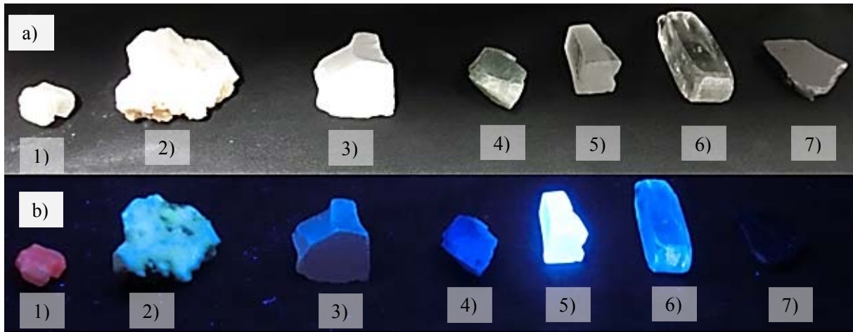
Figure 82: Samples for the recording of luminescence spectra a) under white light b) under 15W excitation with light of 254 nm at a distance of about 10 cm: 1) Calcite, 2) Chalcedony, 3) Magnesite, 4) Fluorite, 5) PbO reference glass 1, 6) CAB 15, 7) Silicon
