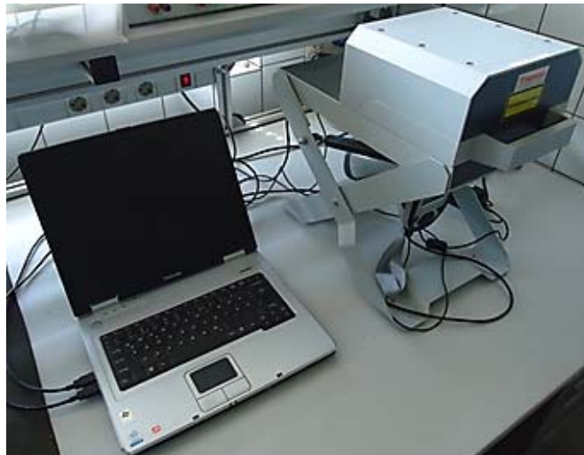
Figure 81: XRF analyzer calibrated with lead crystal of known PbO-content
