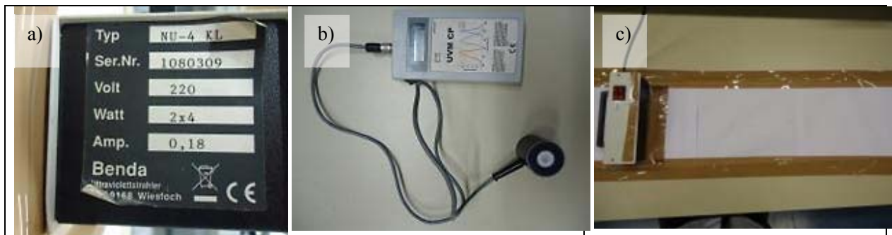
Figure 41: a) The UV-Lamp NU-4 KL, b) UVM CP radiometer, c) experimental setup
