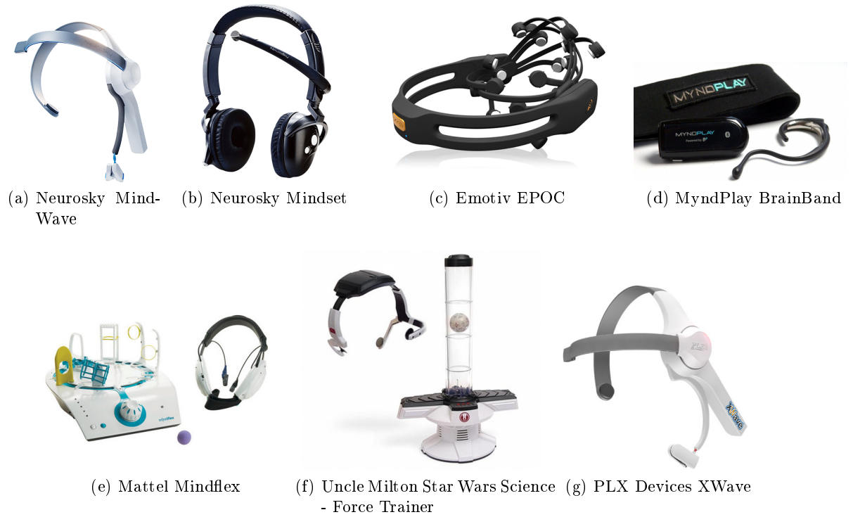
Figure 1.3.1.: A non-exhaustive overview (a–g) of the currently available low-cost consumer EEG devices.
