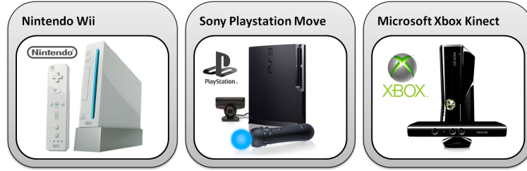
Figure 1.4.1.: Recent input controllers which use a completely different concept for HCI. Although some of the systems still have buttons and joysticks, they focus on body movements to control games.
