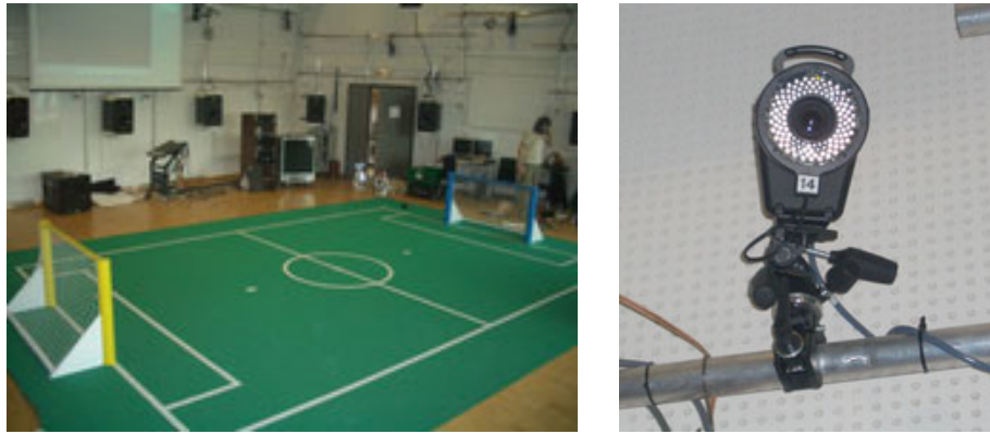
Figure 6.3: Setup for the tracking session. The left image shows the SPL field within the motion tracker system. The right image shows one of the 15 cameras of the body motion tracking system. The LEDs at the front of the camera provide pulsed infra-red light allowing capturing under day light conditions.
