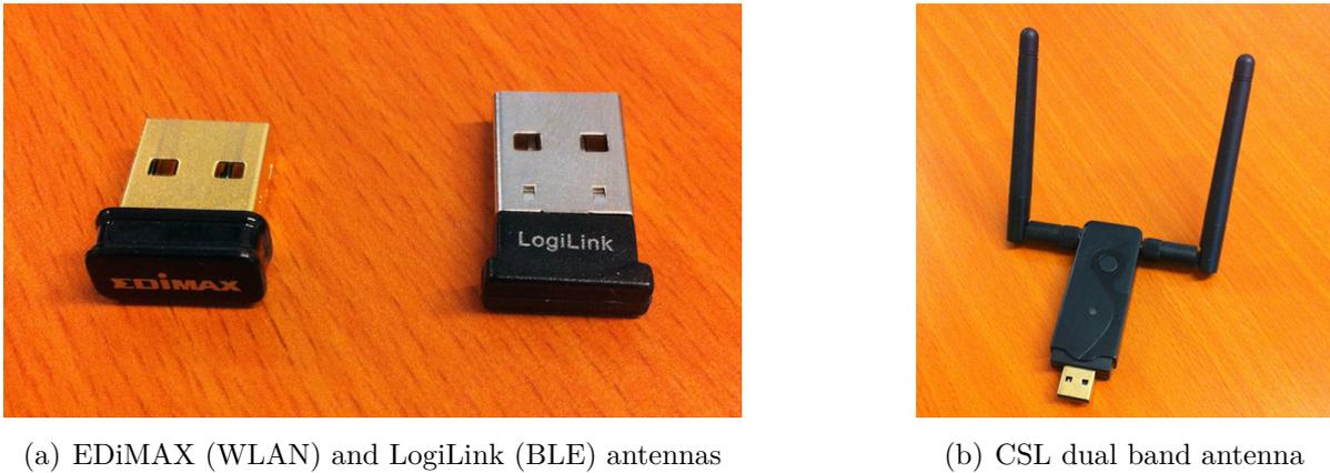
**Figure 4.1:** Used USB adapters for receiving WLAN and BLE data
