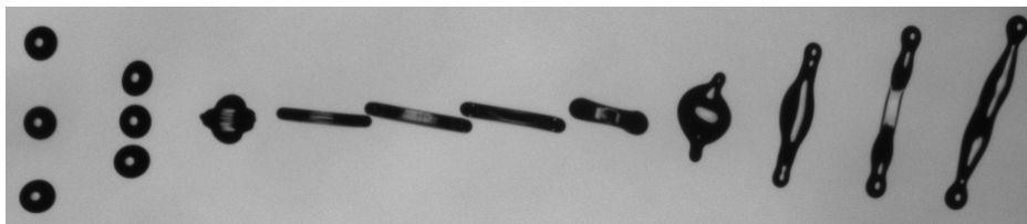
Figure 4.23: Reflexive separation at ternary collision, using glycerol 50% as the liquid, at a large Weber number: D = 399 \mu\text{m} , We = 143.1 , X = 0.11 , f = 5530 \text{ Hz} .
