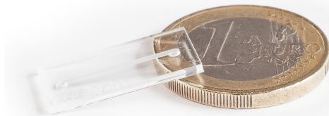
(e) Microfluidic glass chip from iX-factory (thin cover glass); channel width: 1000 \mu\text{m} , channel depth: 300 \mu\text{m}
