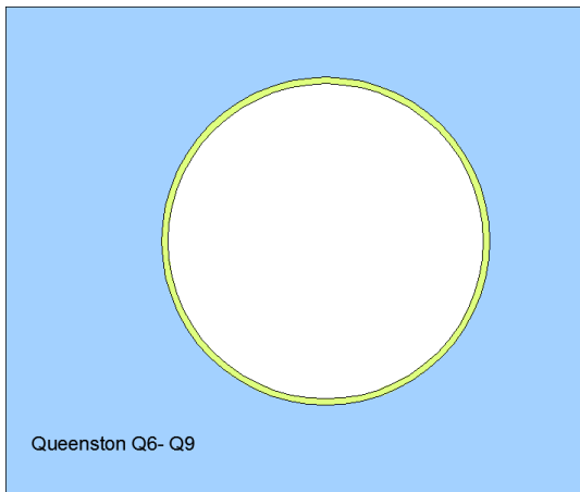
Fig. 15: 2. Activation shotcrete ( M_{stage} = 1,0 ).
