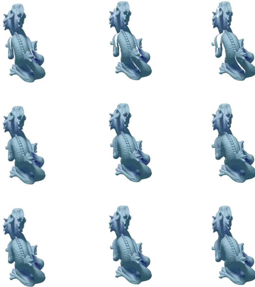
Figure 3.6: Comparison of the two hole filling methods for different warping angles. The first row shows the warped image without hole filling, the second with color interpolation and the third with re-rendering of disoccluded areas.
