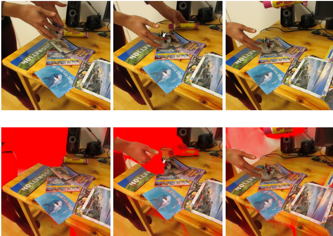
Figure 3.9: Fast motion in the scene. The red areas denote regions where the image registration failed due to fast motion. The fallback to the LR image avoids most artefacts, while some are still visible (e.g. around the yellow and pink glue tube). Results are display in the upper row, confidence map per frame in the lower.
