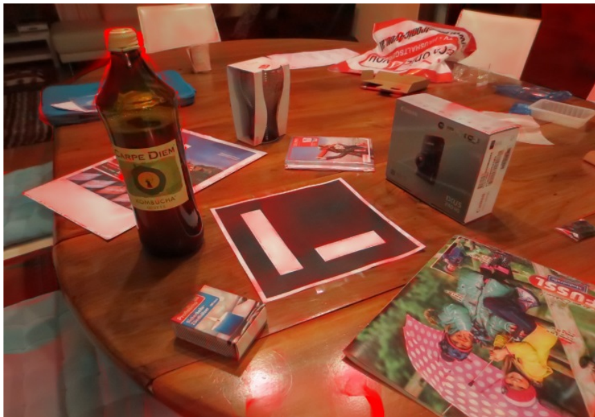
Figure 3.3: Visualization of the confidence map. Red shading denote regions with low confidence like, for example, the area around the bottle which has been disoccluded due to the movement of the camera.
