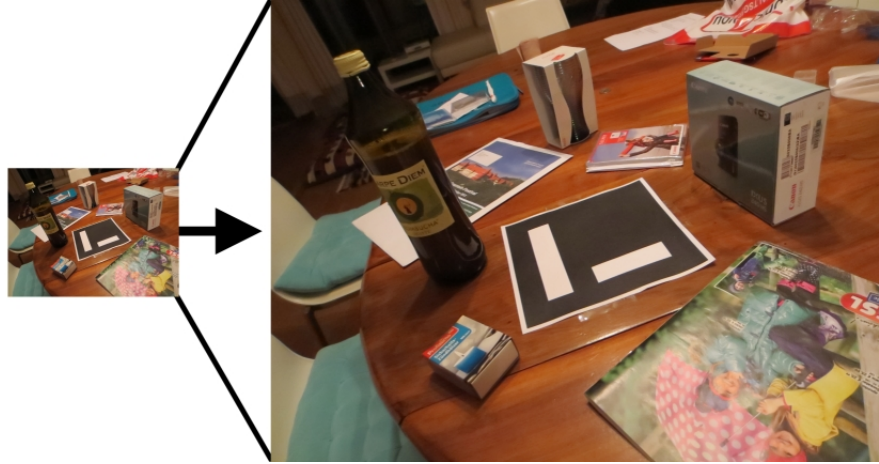
Figure 3.2: Using our method we can upscale a video taken at 640x480 pixel and 30 Hz to 2304x1728 pixel using still frames captured at 5 Hz within 200ms on average.
