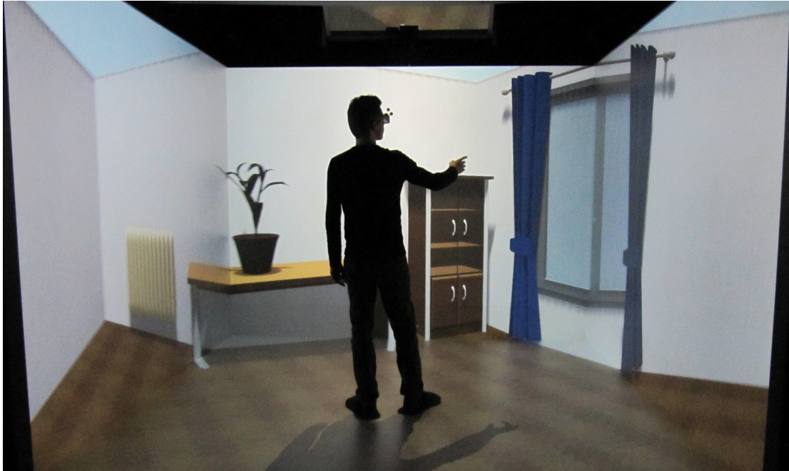
Figure 6.2: The SweetHome3D output is transferred with our web service to an OpenSG CAVE application which lets the user walk through a 3D representation of the house plan [20].
