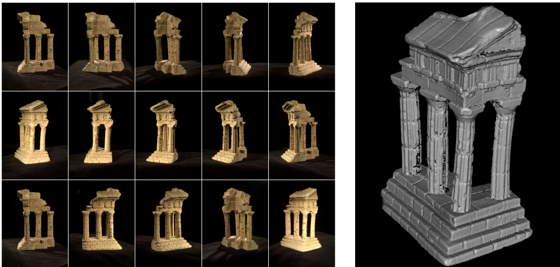
(c) 3D reconstruction: calculate the 3D model from multiple images of the real world object 3
