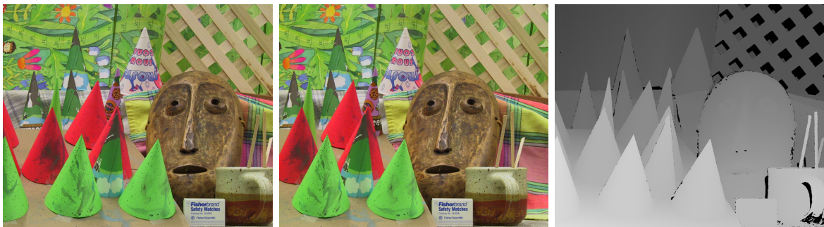
(b) Stereo correspondence: find corresponding pixels in the two slightly different input images. This allows the calculation of relative depth information 2
