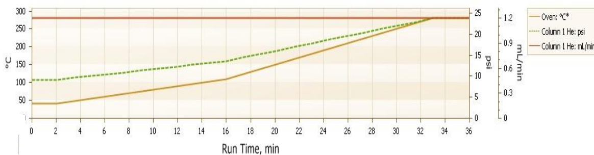
Figure 2.6 – The diagram shows the adjusted temperature gradient in the GC oven. Additionally the carrier gas (Helium) flow is shown, which remains constant while the pressure rises conditioned by the temperature changes.
