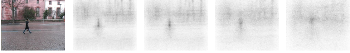
Figure 2.3: Example input image (left), and output of our Hough Forest, i.e. , resulting slices of the Hough space corresponding to different scales. Note, light areas represent low, dark areas high probability for an object center location.
