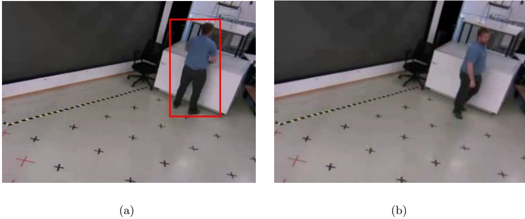
Figure 4.7: Illustration of a problem case for a one shot tracker: The person remains at the position of the first frame annotation (a) while working at the table for some time; (b) when the person finally walks away and thus, its appearance changes, the tracker tends to stick to the background, which exhibits several distinctive image features, to which the part based model has been adapted.
