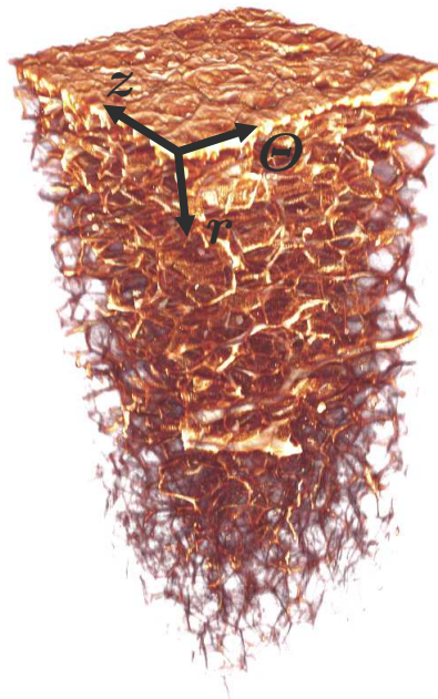
Figure 3.35.: Image stack into the 3-D reconstruction software is shown. One can see very good that the intensity is decreasing toward the r -direction.
