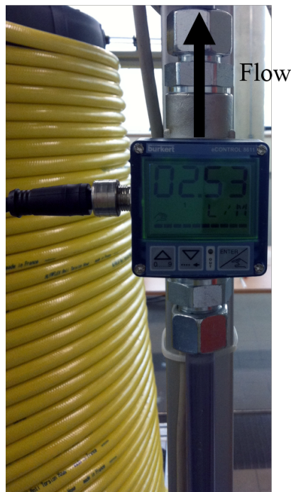
Figure 3-2 PI controller for flow measurement and flow control.
