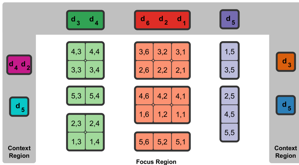
Figure 3.3: The VisBricks Layout: The arch consists of a focus region in the center and two context regions, the arch legs, which only show summary bricks. In the focus region summary bricks are displayed at the top, whereas corresponding segment bricks are added below them.
