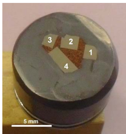
Figure 4-18: Embedded high pressure torsion deformed nickel specimens labeled 1 to 4.
