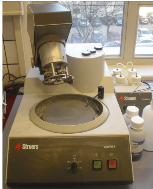
Figure 2-10: The LaboPol5 grinding and polishing machine.
