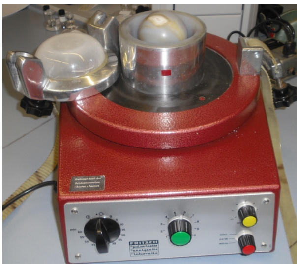
Figure 4-1: Fritsch Pulverisette ball mill.
