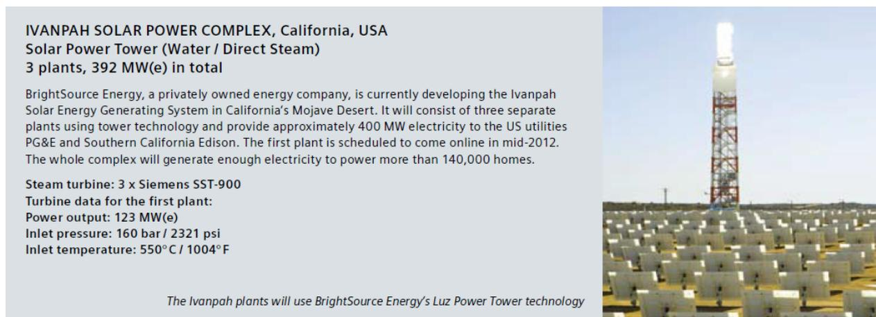
Figure 5-35: Used turbine configuration of the Ivanpah solar tower power plant, California, USA [61]
