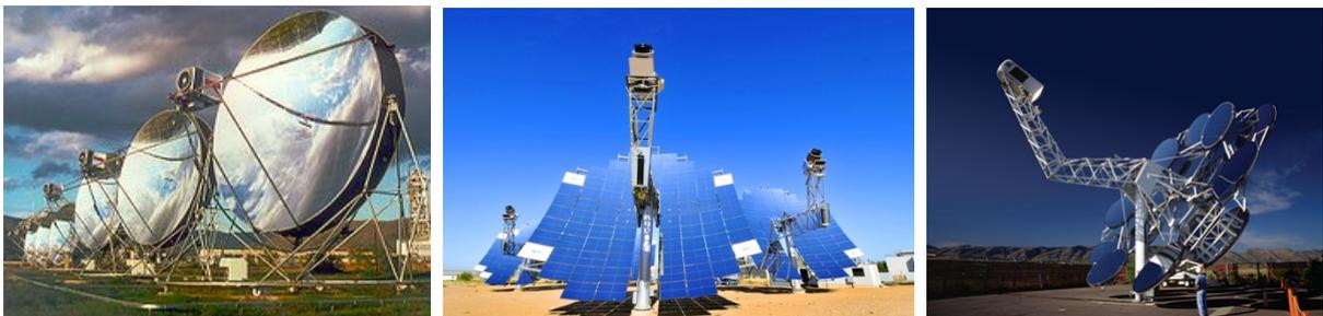
Figure 2-7: Dish Stirling construction types ([74], [76], [53])
