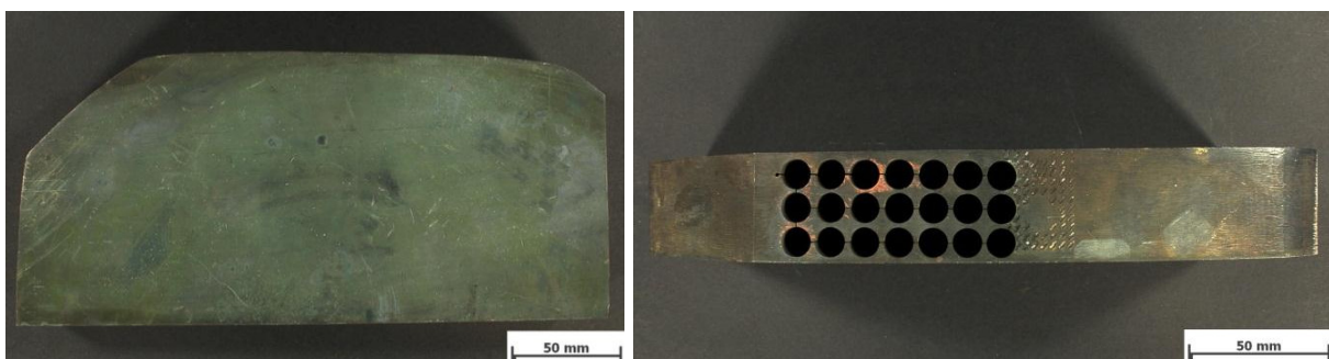
Figure 38. Sampling positions of Haynes 282 tensile specimens
