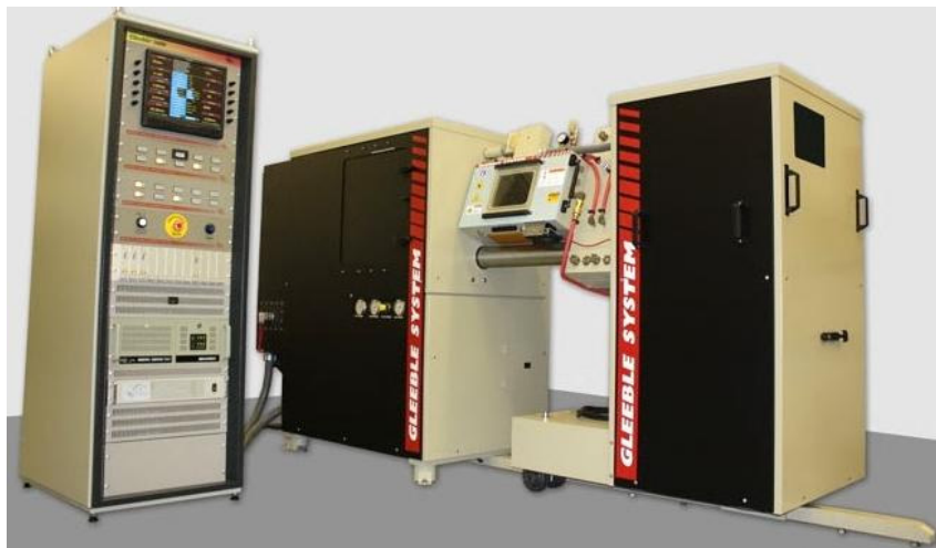
Figure 45. Gleeble 3800 testing system used for thermomechanical testing 82
