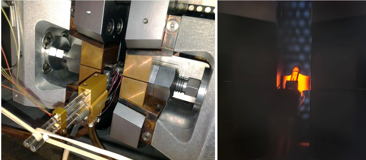
Figure 52. Setup of CGauge sensor (left) for strain determination during thermomechanical testing (right)
