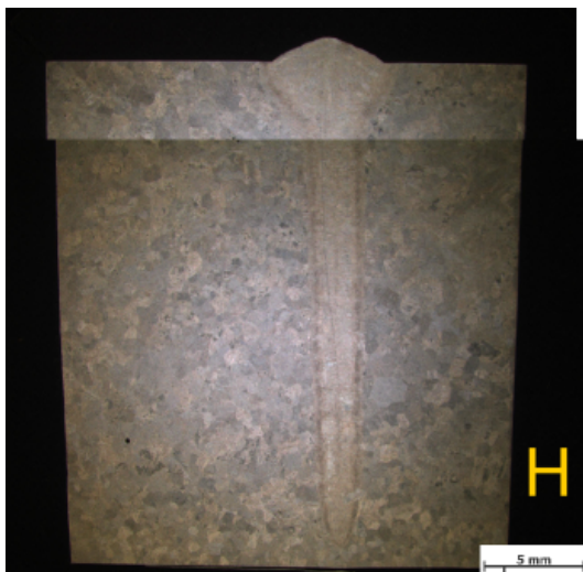
Figure 4.21: WTP,blind weld H [Adler]: cross-section, no pores and not fully penetrating but penetration depth is larger than for E, the overall quality is adequate, regular weld bead
