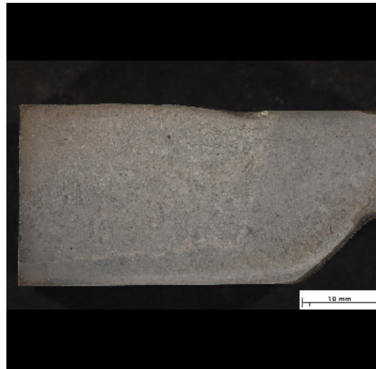
Figure 4.24: WTP, blind weld 7 [Adler]: longitudinal cut, the penetration depth over the weld seam length is not constant, a general decrease is identifiable which starts at the mid of the weld seam and is thus not triggered by the slope-out of 5 mm.
