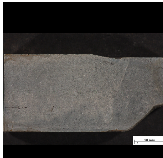
Figure 4.26: WTP, blind weld 8 [Adler]: longitudinal cut, the quality in general is adequate, the etching process revealed despite repeated etching an inhomogenous result. a small crack is visible, the through-welded root is an indication that the plate is fully penetrated.
