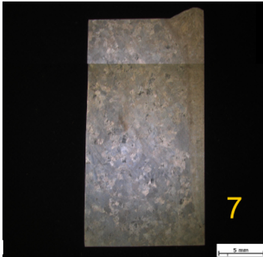
Figure 4.23: WTP, blind weld 7 [Adler]: cross-section, no pores and not fully penetrating, the overall quality is adequate, regular weld bead, the cross-sectional cut was performed after the longitudinal cut.
