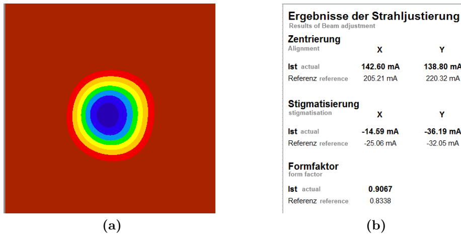
Figure 3.7: Screenshot of the result screen after the auto beam adjustment: the resulting beam profile is displayed in pseudocolor (a) together with the values defined for centering and stigmatisation (b).
