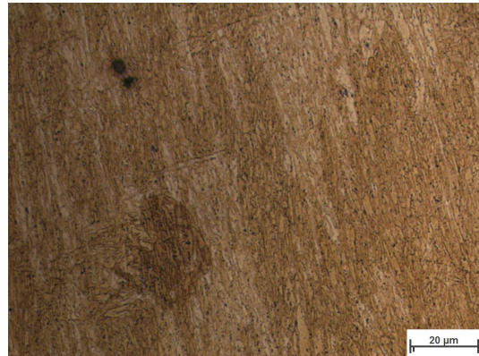
Figure 4.50: Microstructure at the center of the simulated HAZ in as-welded condition, T_{peak} = 1100^{\circ}\text{C} .
