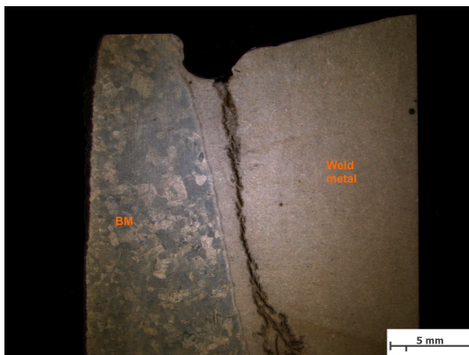
Figure 4.16: MTP, longitudinal section of blind weld E [Adler]: severe end-crater crack due to restraint to shrinkage of the concave shaped weld seam, improper slope-out.
