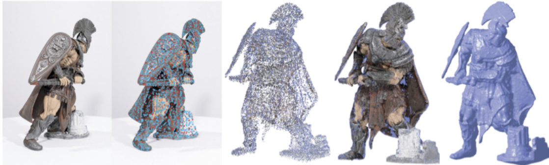
Figure 2.12: Illustration of the entire patch-based multi-view stereo reconstruction process. From left to right: Input image, Harris and difference-of-Gaussians features, reconstructed patches, filtered patches, final mesh model. This set of images are taken from [31].
