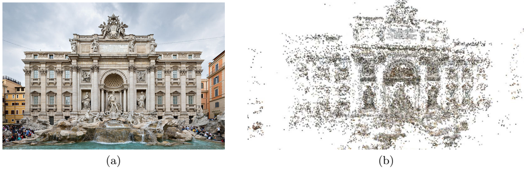
Figure 1.1: a) Photograph of the Trevi Fountain in Rome. b) 3D model of the same object, reconstructed by applying an image-based approach as described in [94, 95]. These images are taken from Wikipedia 3 and [94], respectively.
