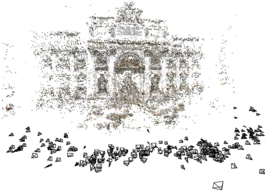
Figure 2.11: Reconstruction of the famous Trevi Fountain in Rome, Italy containing a 3D point cloud and additional estimated camera positions and directions are visualised. This image is taken from [95].
