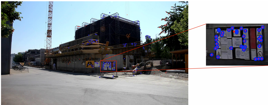
Figure 3.12: Due to the high compression of feature descriptors in several image parts, the estimated camera pose can be extremely inaccurate if several features are selected from the same area of the image.
