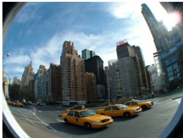
Figure 3.7: New York City seen through a fish-eye lens with a high barrel distortion, which is a type of radial distortion 1 .
