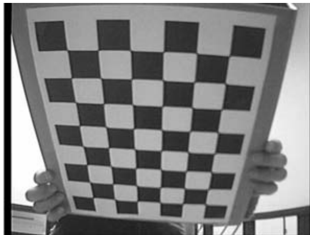
Figure 3.2: Planar calibration target applied to generate training examples for Zhang's model. This image is taken from [97].
