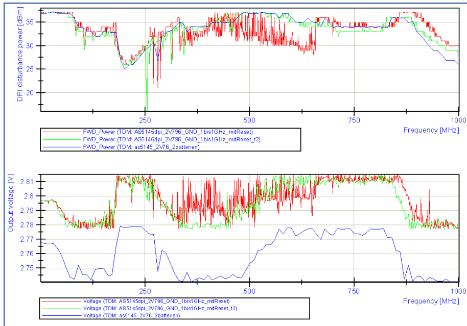
Figure 4.48: as5145 DPI measurement - disturbance coupling to VSS. The three results are obtained by the usage of three different power sources. The first measure (red) was done while using a Agilent E3631A. For the second measurement (green) a Weier Electronics W30 was used. The third measurement (blue) was done using a lead-acid batterie and a linear voltage regulator (LM7805) to provide DC power to the DUT. The last measurement was done with less frequency steps.
