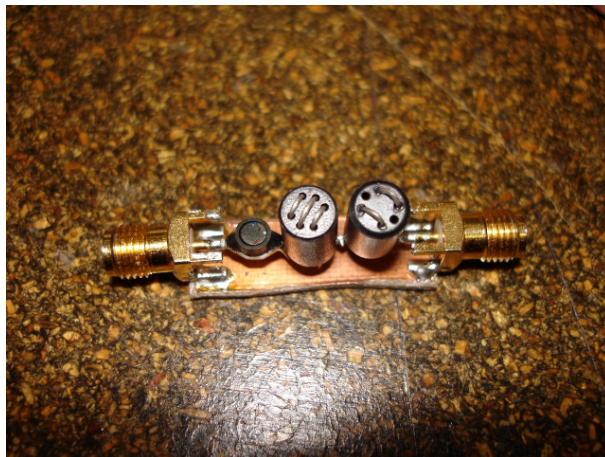
Figure 4.21: Decoupling Network (Fig. 4.6) mounted in a simple Adapter Board, called Probe 1 or Probe 2.
