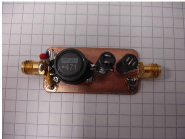
Figure 4.23: Decoupling Network mounted in a simple Adapter Board, called Probe 3.
