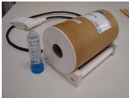
Figure 3.2.: 1H Transmit / Receive Volumen Coil for mice and a Falcon Tube used for phantom and preclinical experiments.
