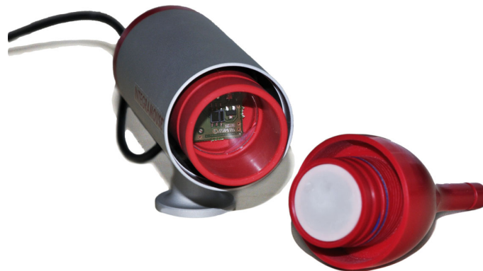
Figure 2.6: Opened IntegraMouse ® showing the control unit and the membrane placed between mouthpiece and controller.
