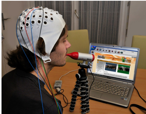
Figure 2.1: System setup consisting of the user wearing the EEG-cap, the IntegraMouse ® and one single PC running the Qualiworld application as well as the Simulink model of the Fusion and the SignalServer.
