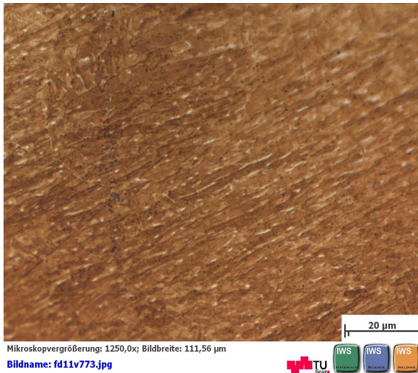
Figure 10: CB2A quenched at 1250°C.
