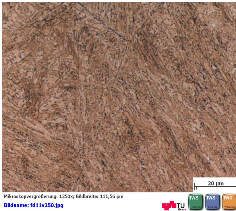
Figure 31: NPM1 quenched at 1050°C.
