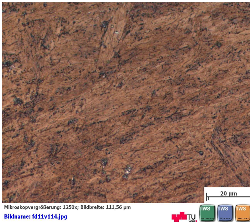
Figure 43: NPM1 quenched at 1046^\circ\text{C} .
