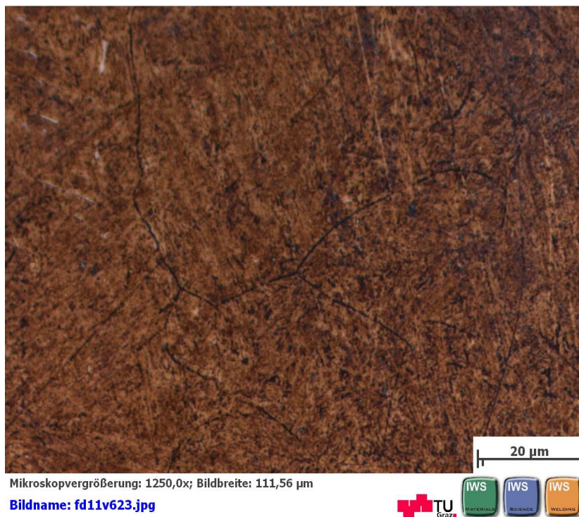
Figure 20: CB2A quenched at 730°C.
