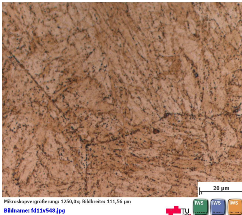
Figure 40: NPM1 quenched at 730°C.
