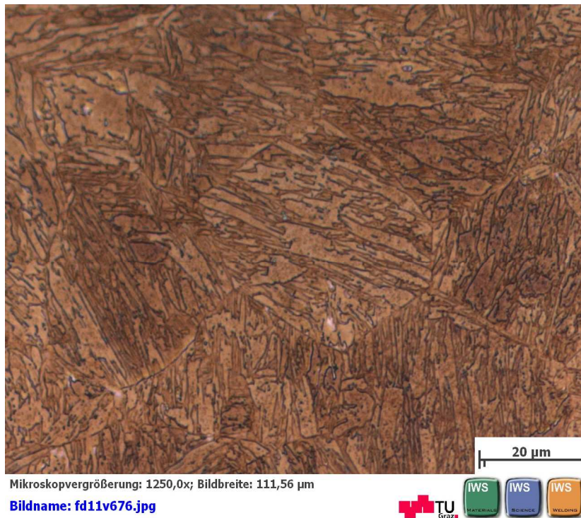
Figure 51: NPM4 quenched at 1200°C.
