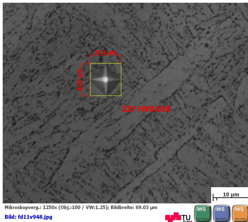
Figure 58: Hardness micrograph of NPM1 in the as-received condition.
