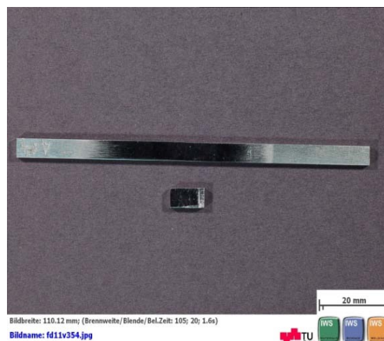
Figure 7: Applied dilatometer samples of the CB2A -Heat 145 material.
