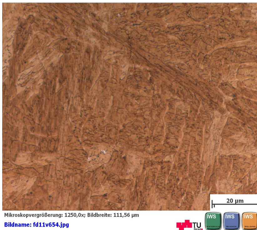
Figure 11: CB2A quenched at 1300°C.
