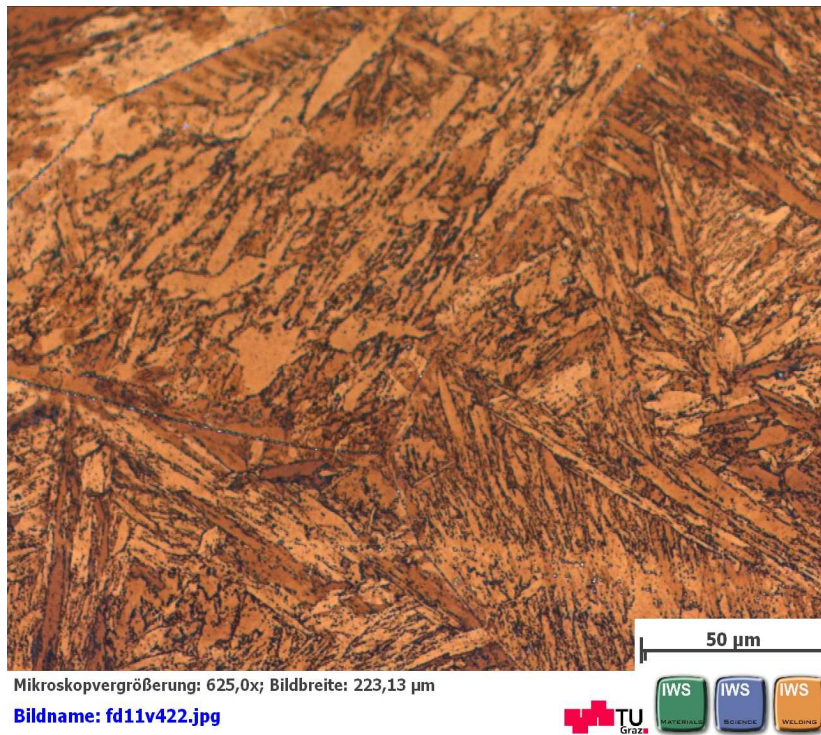
Figure 47: NPM4 quenched at 900^\circ\text{C} .
