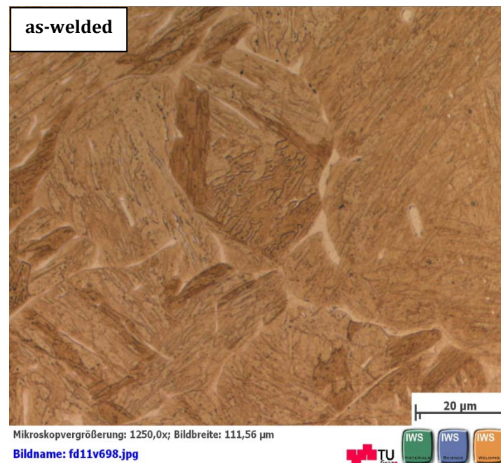
Figure 27: Optical micrograph of NPM1 in the as-welded condition with a heating and cooling rate of 10 K s -1 .
