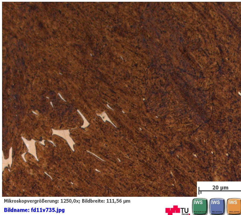
Figure 19: CB2A quenched at 650°C.
