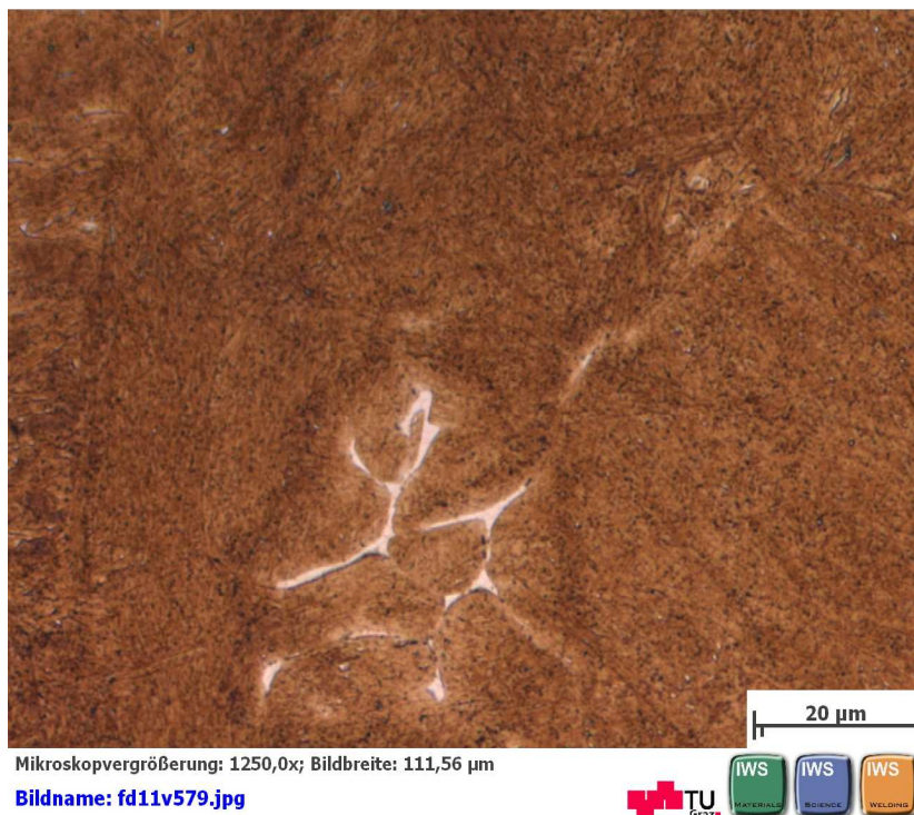
Figure 18: CB2A quenched at 600°C.
