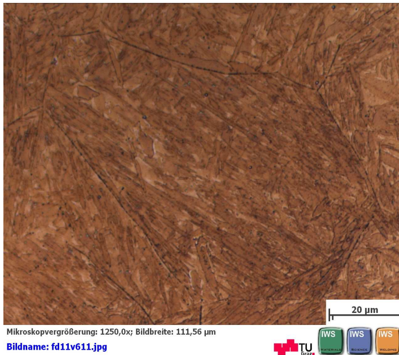
Figure 26: CB2A quenched at 1196°C.
