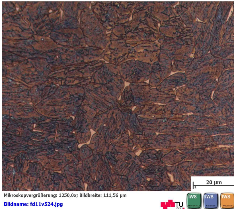
Figure 16: CB2A quenched at 580°C.
