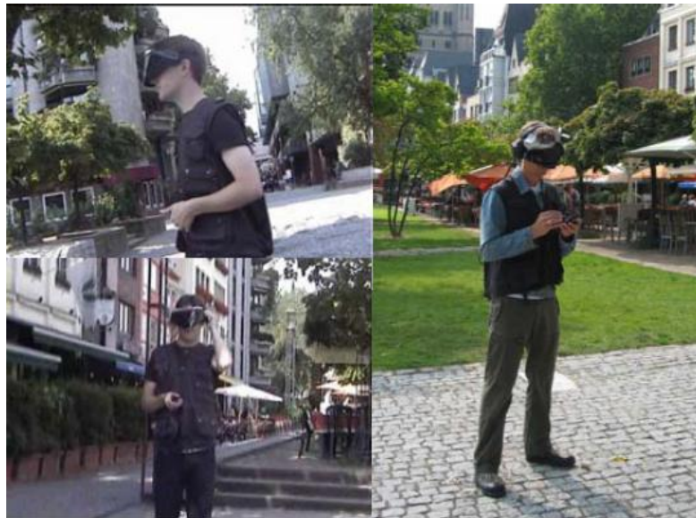
Figure 7: The setup used for TimeWarp [9]. The user is wearing goggles which display the VR objects and is using a PDA which is used to navigate around the city and solving the riddles
