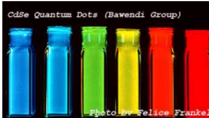
Figure 2.3: Fluorescence emission of CdSe-nanocrystal solutions, with increasing crystallite size from 20 Å to 80 Å [18].
