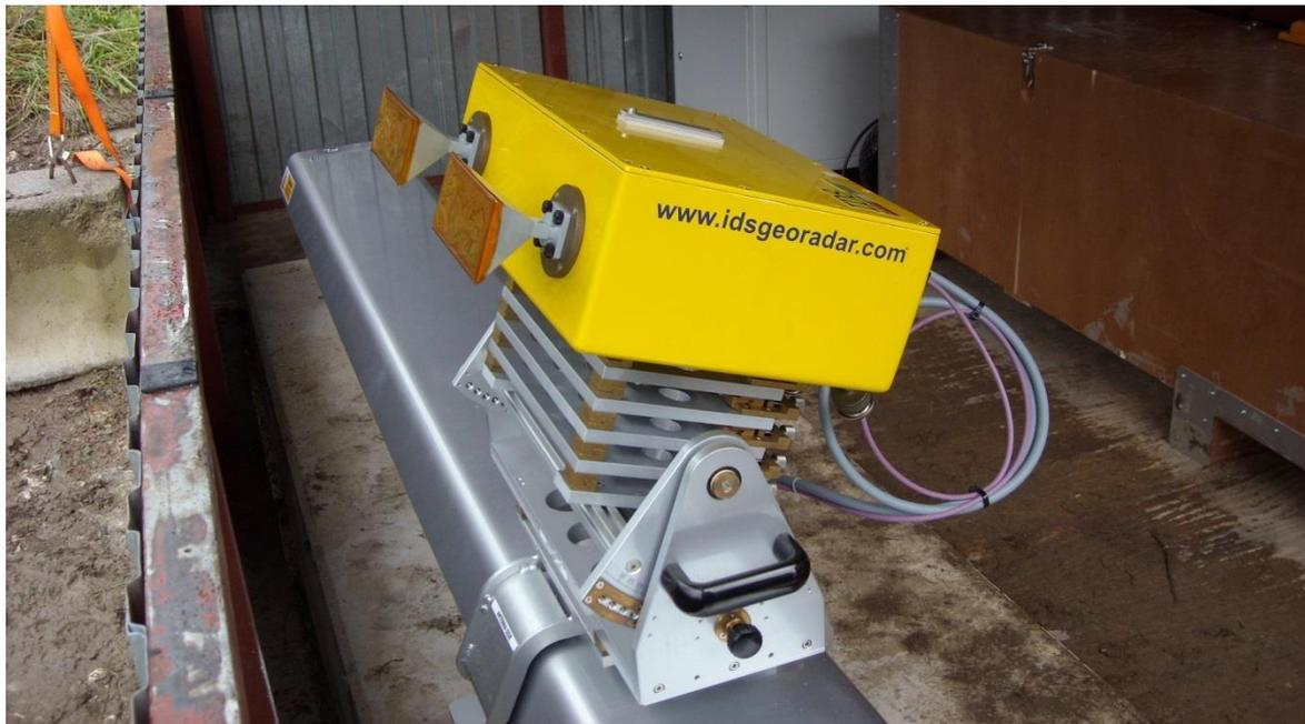
Figure 34, The tilted radar head mounted on the 'elevation pointing system' using several spacers for ideal positioning.
