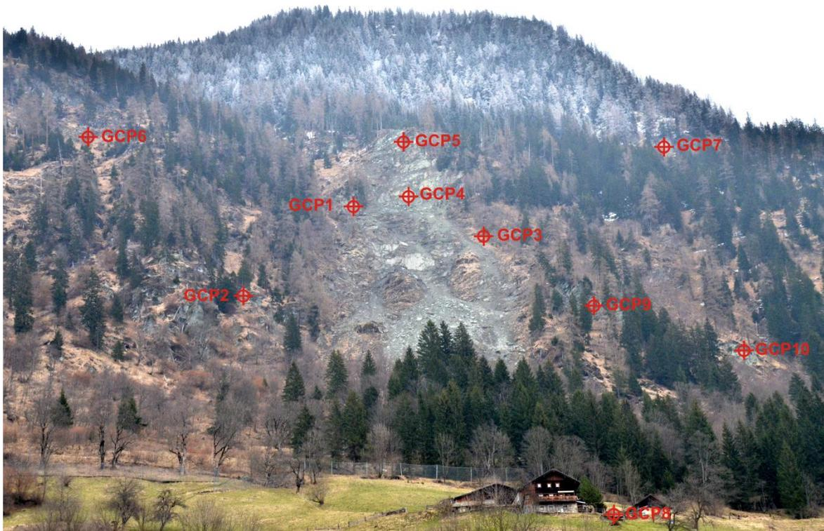
Figure 61, Position of all 10 Corner Reflectors within the investigation area.
