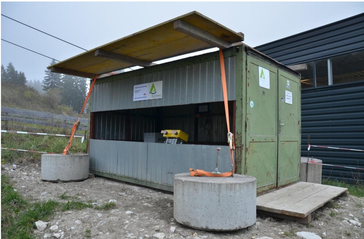
Figure 39, Completely installed IBIS-FL radar at Reutte within the equipment shelter.
