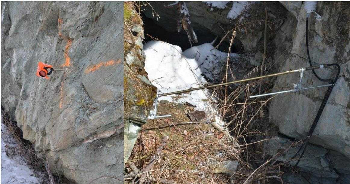
Figure 31, Fixed reflecting prism at the upper part of the Ingelsberg; Installed fissurometer inside one of the major cracks at the top of the Ingelsberg
