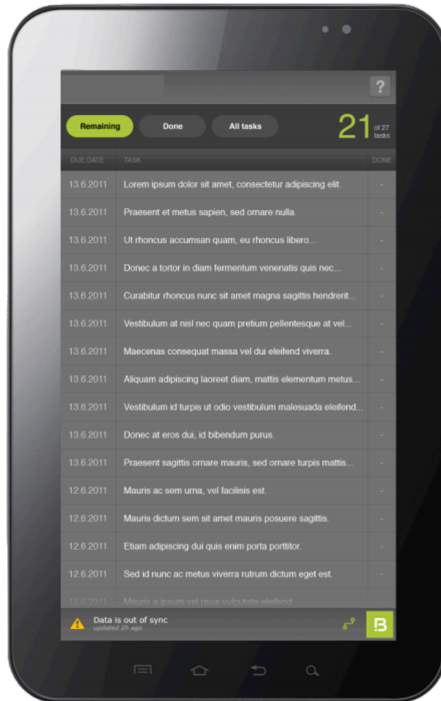
Figure 4.4: A list of maintenance tasks in the first version of the Boom Mobile app. Note that the height of a single entry is rather low, making it hard to select.
