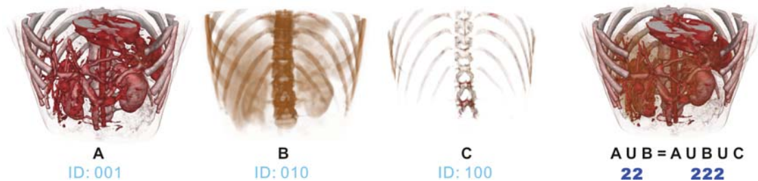
Figure 6.1: Volume Clipping of medical Liver Data. Three volumes uses the same volume data set and different transfer functions
