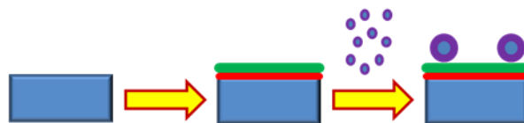
Figure 45: Layer by layer with polysaccharides and C.A. nanoparticles. The first block is a model surface without any coated substances, the second block contains the polymers which are introduced on the surface by LbL-technique, and the third block shows the polymer coatings with adsorbed active compounds like enzymes on it.
