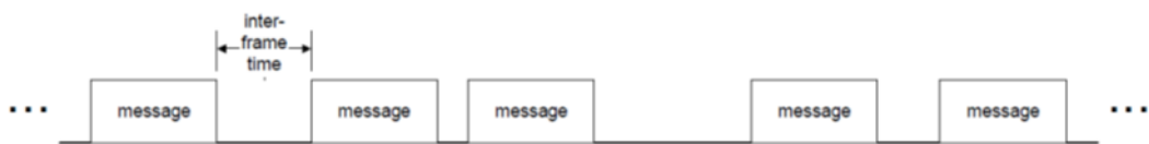
Figure 29: Timing of Test Message
