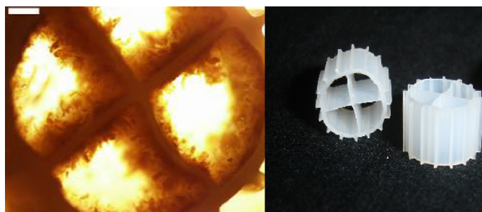
Figure 1.12: Enlarged Kaldnes K1 carrier with biofilm (left) and two Kaldnes K1 carriers in real size (right) [18].
