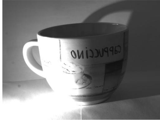
Figure 3.7: Scene with illumination artefacts. Due to illumination artefacts the scene produces a wide range of brightness variations. It is not possible for the image sensor to capture this high dynamic range.
