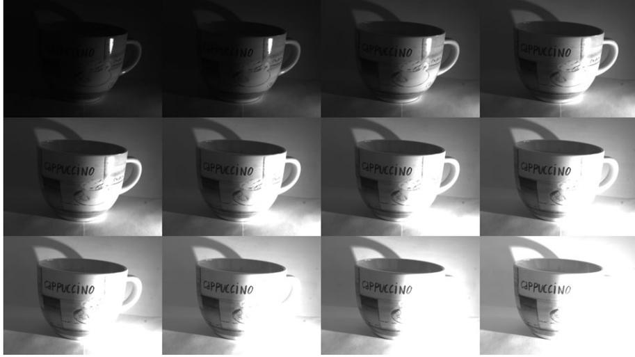
Figure 3.9: HDR Grayscale photographs. Twelve images of an sample scene with different exposure times  $\Delta t$  are acquired for calibrating the response function  $g$ .
