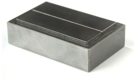
Figure 6.15: Planar Specimen. Object with two defined planes in  $1\mu m$  height difference.
