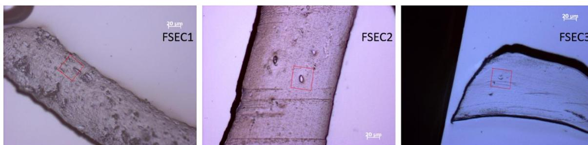
**Fig. 28:** LIMI images of FSEC1 (left), FSEC2 (middle) and FSEC3 (right) samples. The red squares indicate the area for the subsequent characterisation experiments via Raman spectroscopy.
