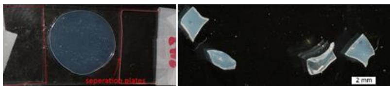
**Fig. 24:** Drying of the gel between glass slides (left) and resulting stiff flakes after the fractional solvent exchange (right). [3]
