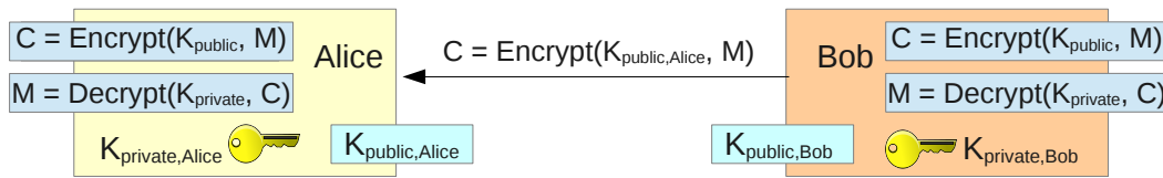
Figure 2.2.: Basic concept of asymmetric cryptography: Alice and Bob each have a key pair of their own. Bob uses Alice's public key for encryption, who in turn can decrypt using her private key.
