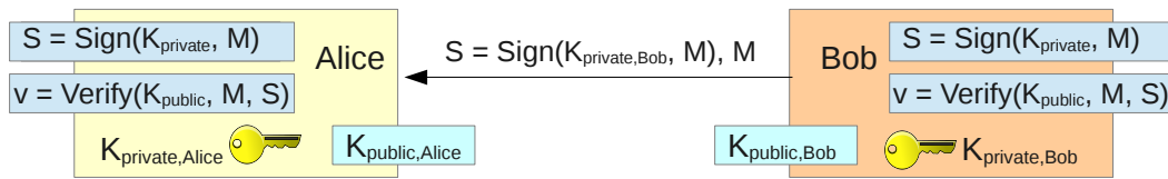
Figure 2.3.: Using asymmetric cryptography for signatures: Alice and Bob each have a key pair of their own. Bob uses his private key for signing a message. Alice can verify the authenticity of the message using the signature and Bob's public key.
