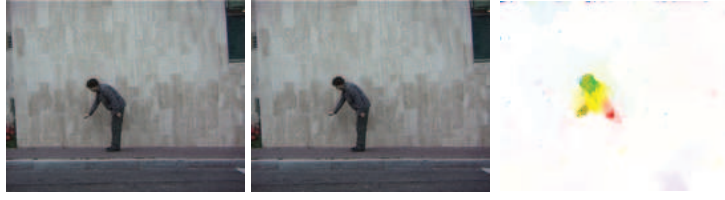
Figure 3.1: Example of flow field - (left) the two input images (right) the computed flow field between those. For visualization purposes the angle of the field is encoded in the colour value whereas the magnitude in its saturation.
