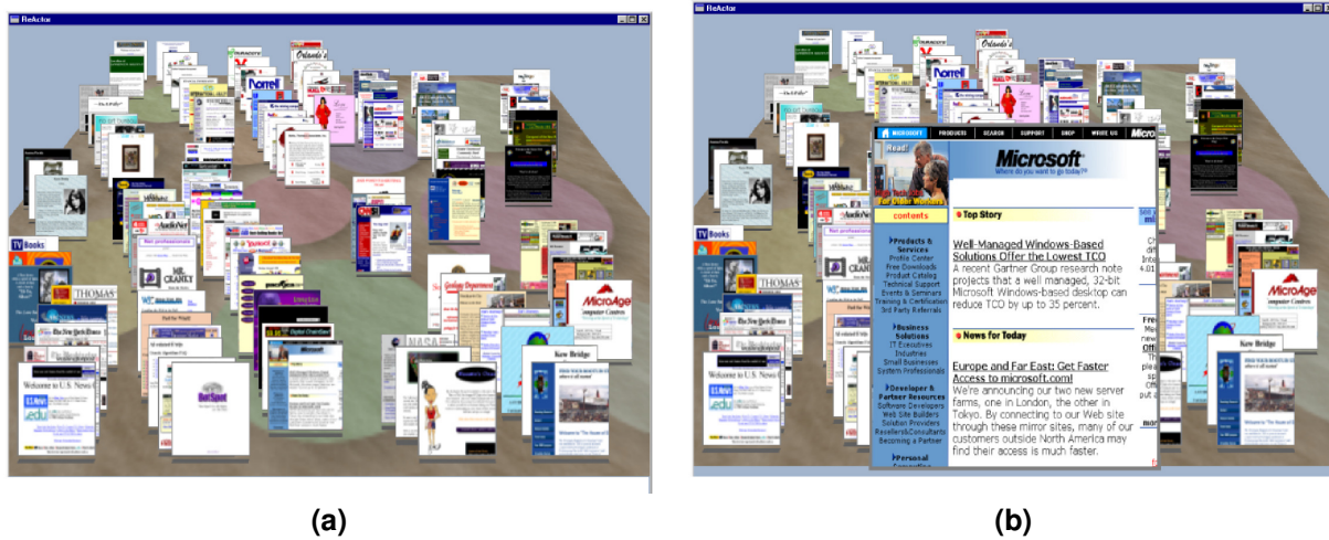
Figure 2.29: (a) The DM consisting of a tilted and textured plane with 100 thumbnails. (b) The DM with a thumbnail in the preferred position. Images from [73].
