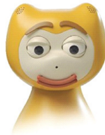
Figure 3.2.: The social feedback agent iCat from Midden and Ham [40] gives feedback through facial gesture
