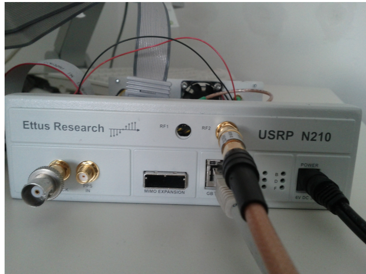
Figure A.2.: Front view of the USRP N210
