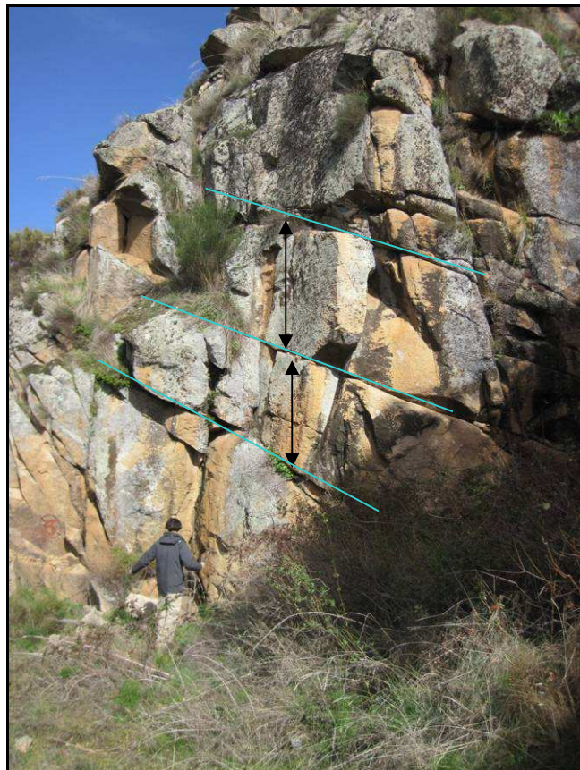
Fig.6 22: Outcrop at the left side of the river. Intense jointing of the rock resulting in the formation of blocks. Spacing (arrows) is well visible in this picture. Lines indicate joint set 5. Person for scale in front.
