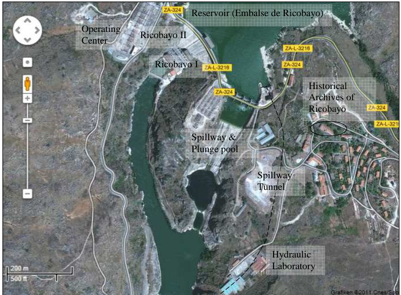
Fig.5 2: Satellite image of the Ricobayo Dam facility. Labeled are the most important features related to the dam (modified after Google Maps, 2012).
