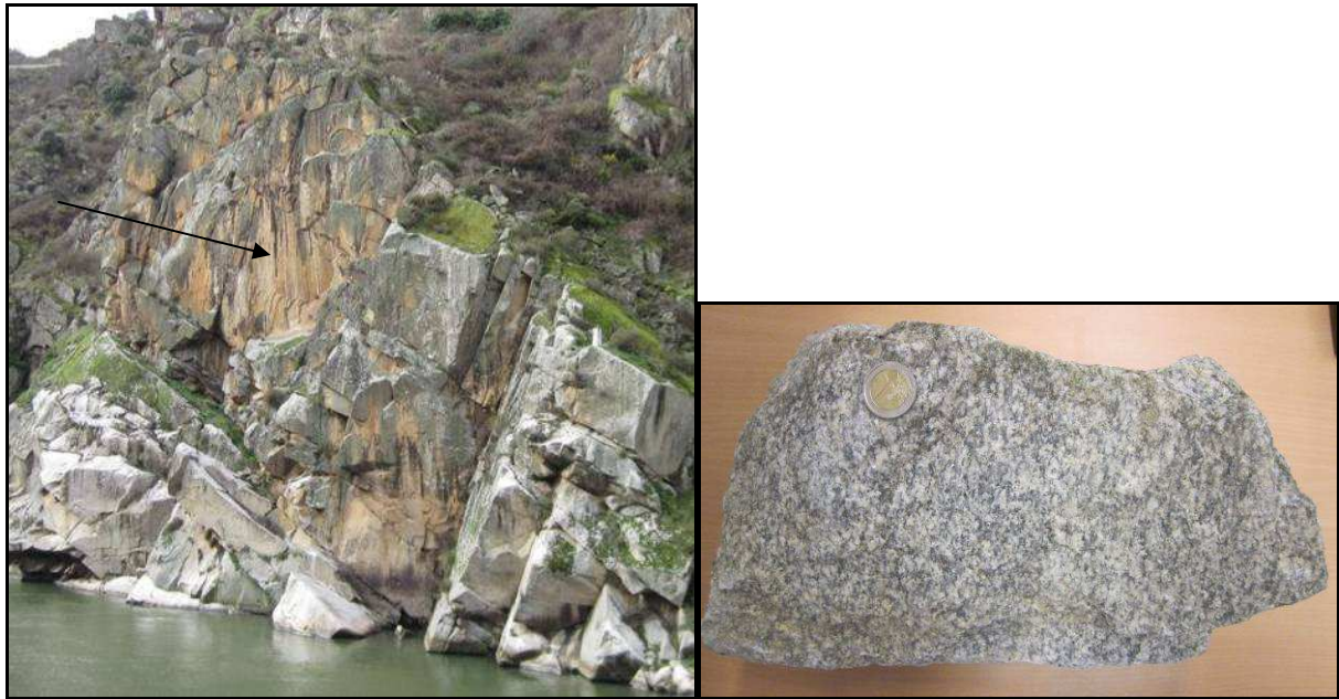
Fig.6 19: Outcrop of the granodiorite of Ricobayo with iron oxide altered surfaces(arrow) (left). Hand specimen of the granodiorite (right). The rock is mostly composed of Quartz (grey) and Plagioclase (white), Potash feldspar (reddish) and Biotite (black). 2€ coin for scale.
