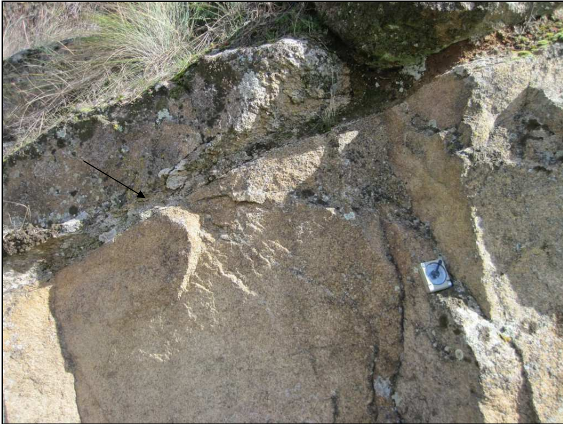
Fig.6 32: Filling of joint (~3cm wide; arrow) along joint set 1. Slightly reddish discolorations on vertical rock wall. Compass for scale.
