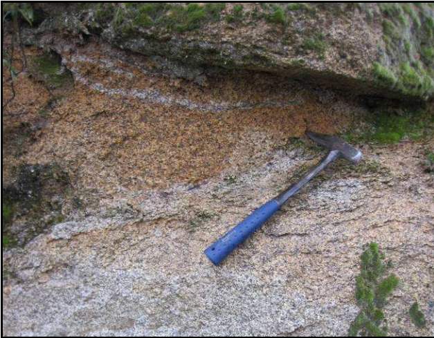
Fig.6.28: Picture showing a strongly weathered rock (R0 to R1). Geologic hammer could be indented without great effort and ripped by hand.
