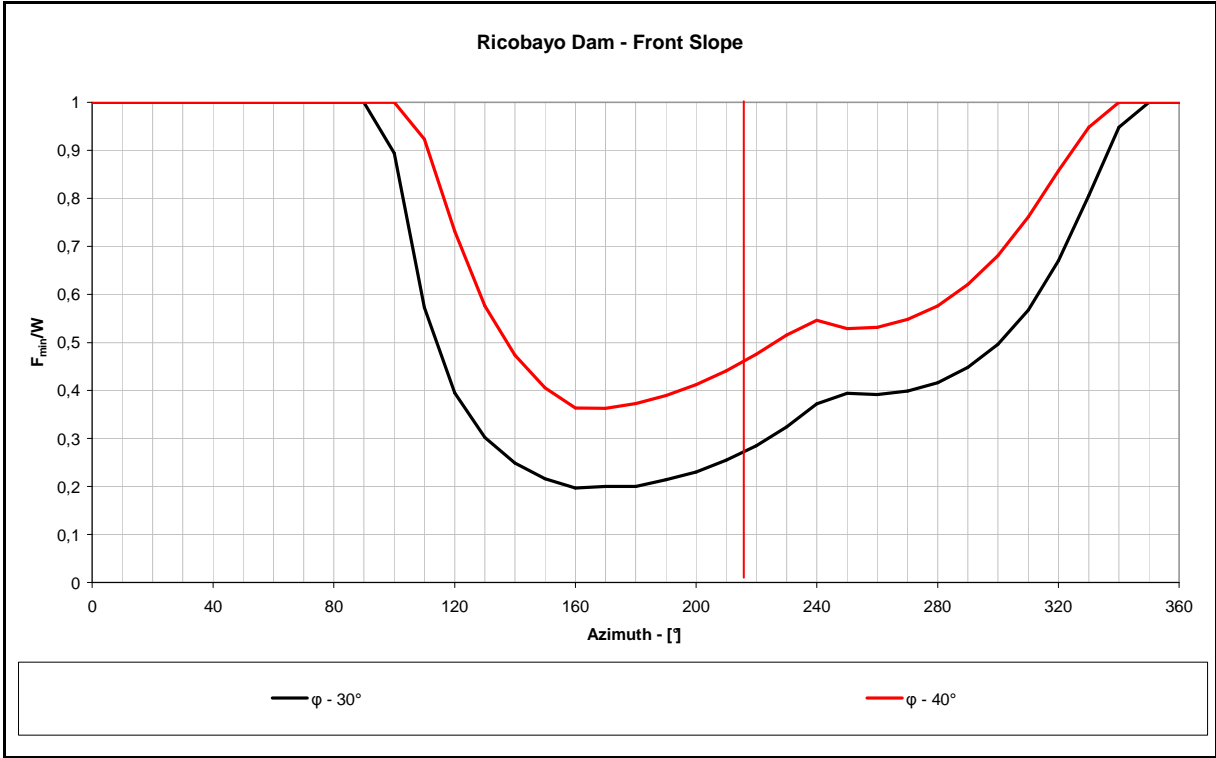
Fig.7 24: Minimal force envelope for the front slope for friction angles of 30° and 40°. The spillway flow is indicated by vertical red line.
