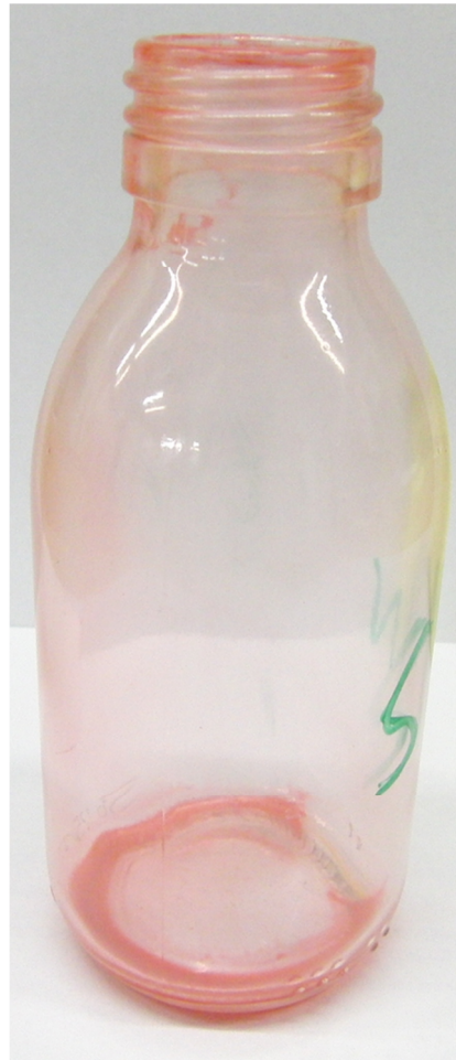
Figure 10-15: Sample N - bad coating
