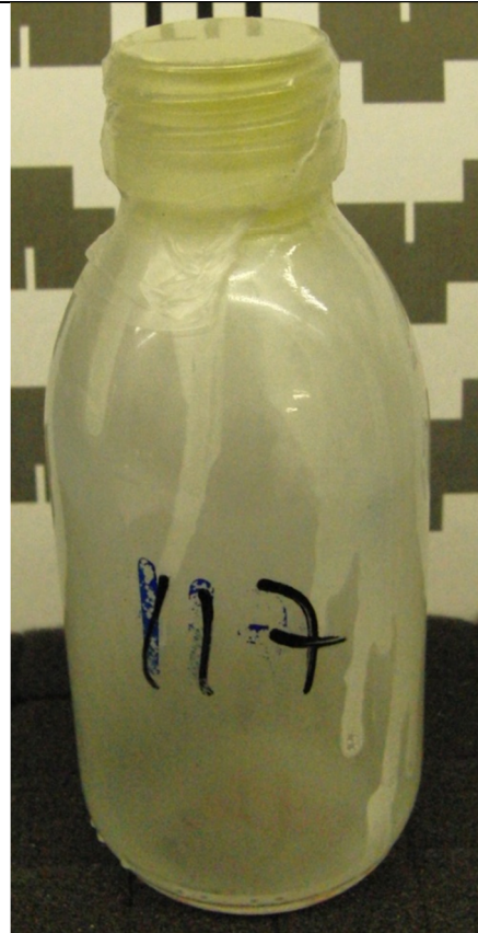
Figure 10-41: sample 117 (9 sec 10% w/w \text{Ti}(\text{iOPr})_4 at 65^\circ\text{C} ; p=5\text{bars} )
