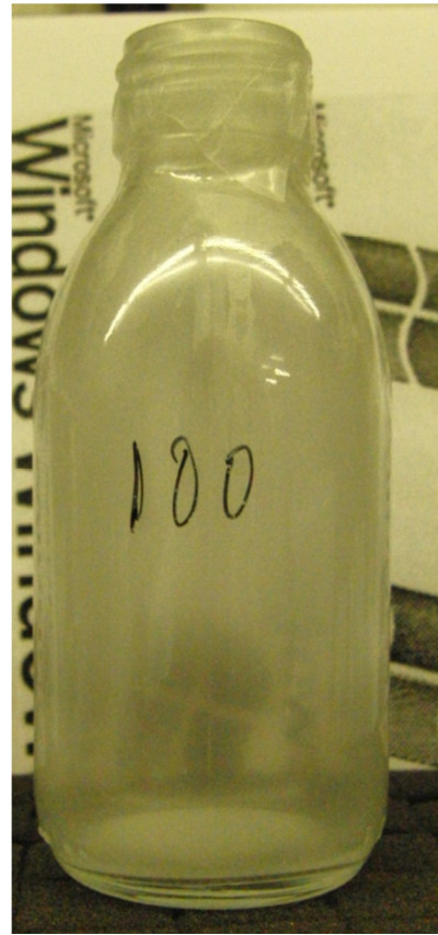
Figure 10-39: Sample 100 (7 sec 10% w/w \text{Ti}(\text{iOPr})_4 at 100^\circ\text{C} ; p=4\text{bars} )
