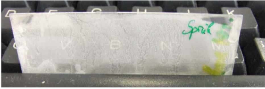
Figure 10-5: unwashed, concentration of coating solution is 10% w/w
