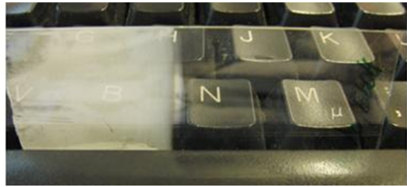
Figure 10-1: Treated, but unwashed slide. The slide was degreased with acetone and ethanol, the left part was coated with titanium dioxide.
