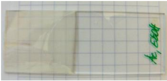
Figure 10-1: Treated, but unwashed slide. The slide was degreased with acetone and ethanol, the left part was coated with titanium dioxide.
