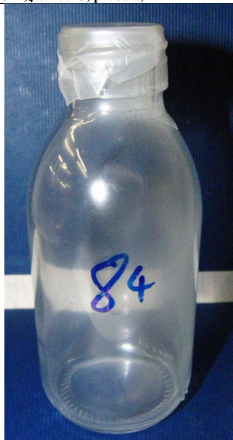
Figure 10-37: Sample 84 (6 sec 10% w/w Ti(iOPr) 4 at 100°C; p=4bars)
