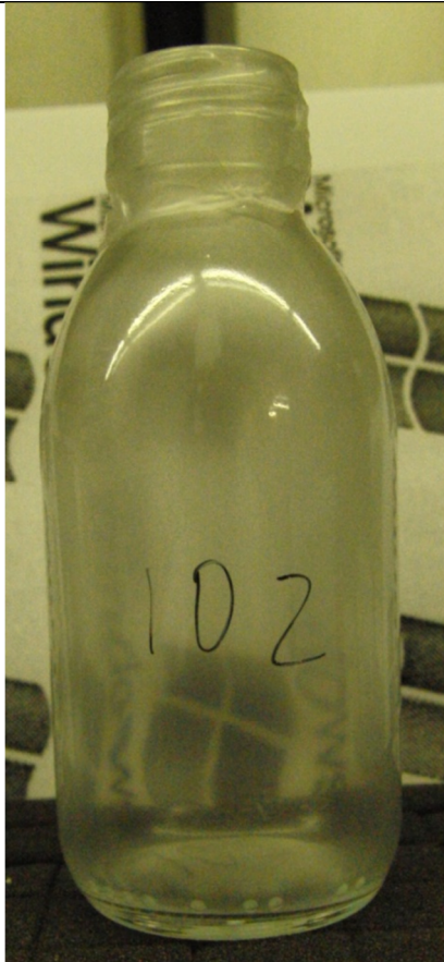
Figure 10-38: Sample 102 (3.5 sec 10% w/w \text{Ti}(\text{iOPr})_4 at 100^\circ\text{C} ; p=4\text{bars} )
