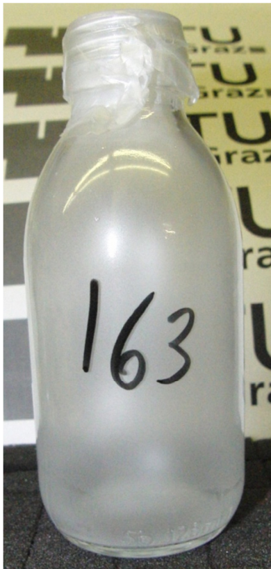
Figure 10-40: Sample 163 (6 sec 10% w/w \text{Ti}(\text{iOPr})_4 at 60^\circ\text{C} ; p=5\text{bars} )
