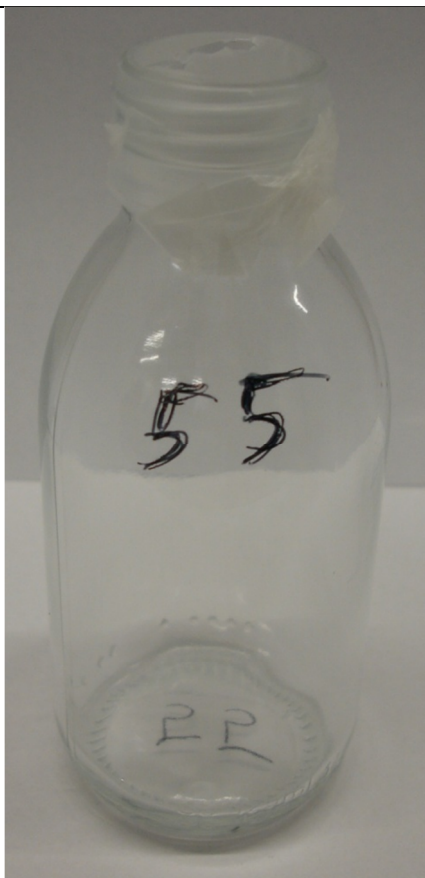
Figure 10-36: Sample 55 (15 sec 10% v/v Ti(iOPr) 4 at 100°C; p=5bars)
