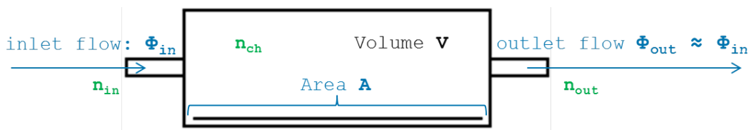
Figure 1: Schematic view of zero-dimensional reactor model (also known as Continuously Stirred Reactor approximation (CSTR)) (after [6]). n_{in} , n_{ch} and n_{out} are the precursor densities at the gas inlet, in the chamber and at the gas outlet, respectively. A marks the area where deposition with a surface reaction rate constant K_s takes place.
