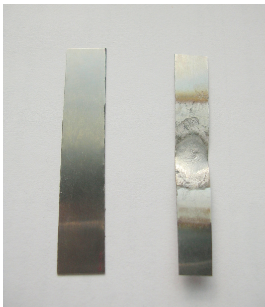
Figure 4.2.: Tungsten strips used for first experiments. Located on the left is the new strip while the one on the right has been fired several times containing steel samples. The remains are not separable of the tungsten anymore and its surface has become rather brittle. One can notice the well which developed due to thermal expansion, weakening during forming of the alloy and of course gravity. Also some tungsten oxide is visible near the ends of the strip where temperature is not high enough to evaporate it.
