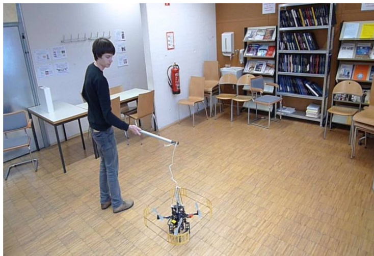
Figure 4.13: Safety feature for testing and tuning the position controller. The fishing rod is a back-up in case of an emergency shutdown.
