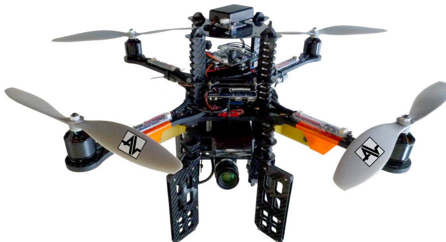
Figure 3.3: Asctec Pelican quadrotor helicopter with a stabilized industrial camera as payload.
