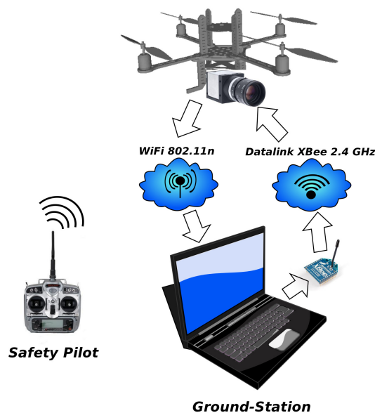
Figure 3.5: Connection interface. The MAV captures the images and streams them via WiFi to the ground-station. The ground-station computes the current pose based on the images and controls the MAV using a wireless datalink. The safety pilot can take over control anytime with the RC.
