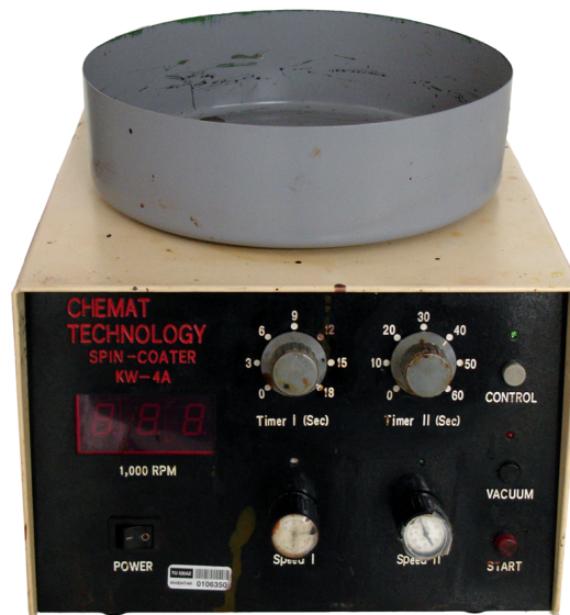
Figure 4.13: Spin coater from Chemat Technology (model: KW-4A ) used inside the flow box;
