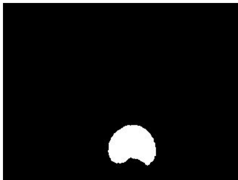
(a) Pixels, where the difference between the old and new depth image is greater than a threshold, are marked as belonging to a motion feature (white).
