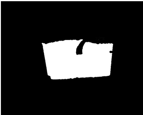
(c) All pixels in the wanted hue range are marked as belonging to a color feature (white). Then the morphological operators are used to remove areas too small.
