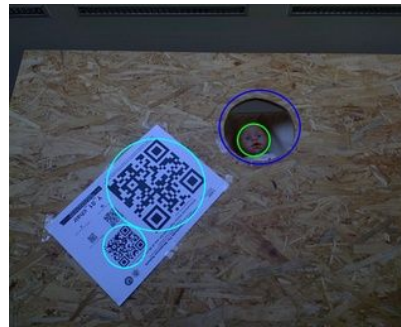
Figure 5.6: Features detected with the Kinect. The color of the ellipse determines the feature type.
