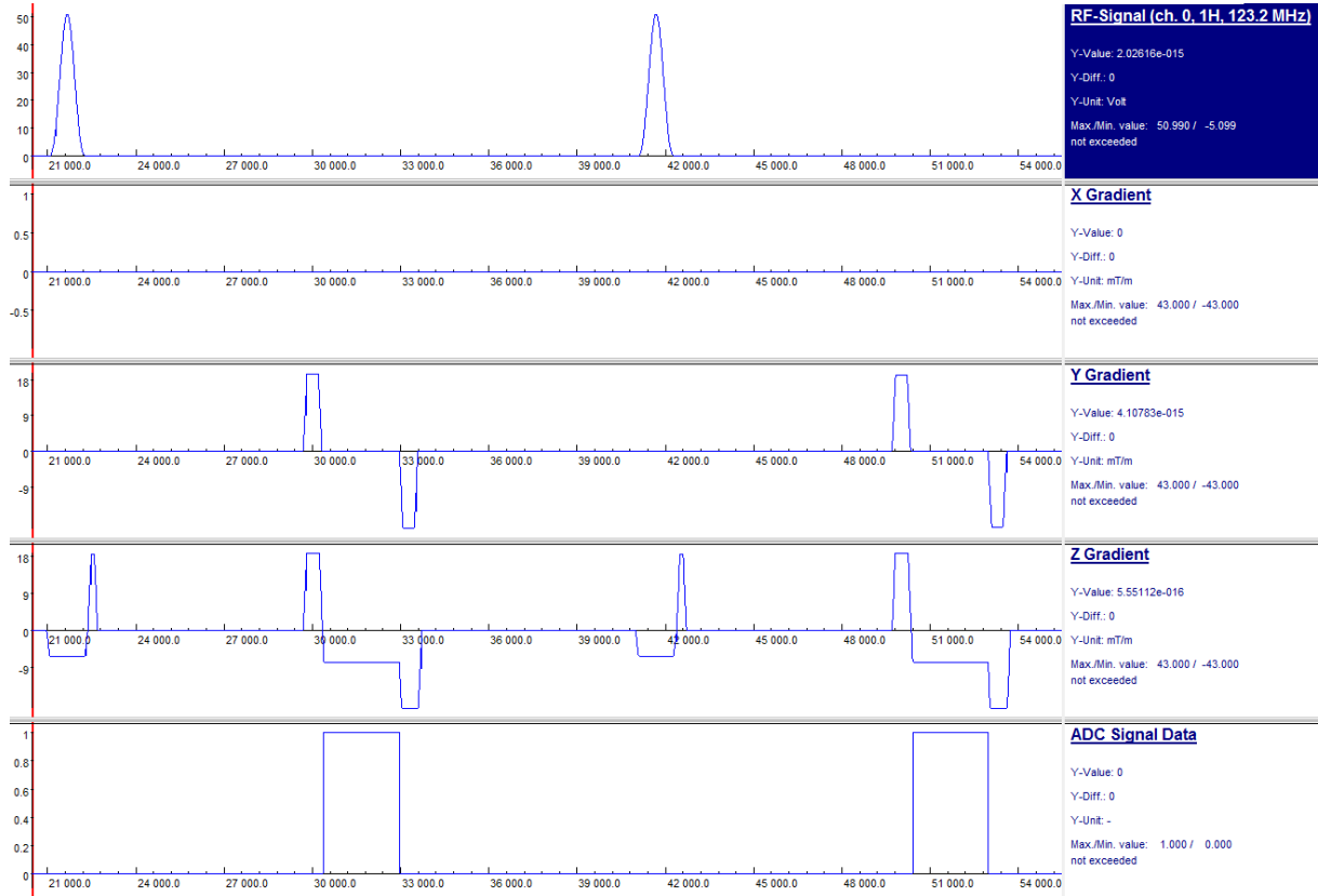
Figure 3.6: Sequence diagram for a GRE based sequence to measure the intensity profiles along the slice direction over two TR-periods. To achieve this, the readout and slice selection gradient are applied in the same direction. Furthermore, the same RF-pulse is used as in the TrueFISP_CV sequence. The diagram was generated by the sequence development environment MultiIDEA in the version VD13.
