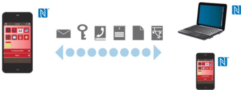
Figure 2.3: NFC Communication: Peer to Peer mode [LTD]
